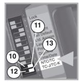
Connect the probe to the input (U). Press MODE, until the desired probe symbol (7) appears. The probe temperature is shown in the lower part of the display (6). The real time infrared temperature is shown in the main display (3).
