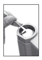
Cleaning the Housing: To clean the exterior housing, use soap and water or a mild commercial cleaner. Wipe with a damp sponge or soft rag.
